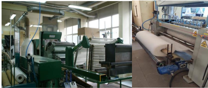
Figure 1. Installation for producing nonwovens using needle punching method
