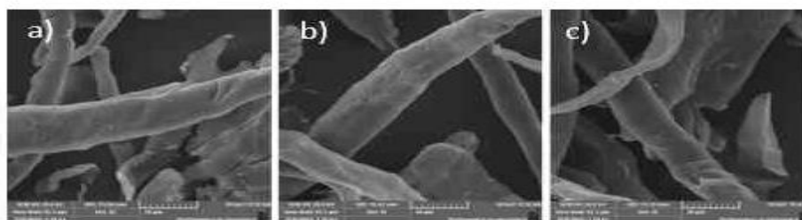
Fig. 4: SEM images of unmodified cellulose (a), modified cellulose CEL_Si69 (b) and CEL_APTES (c) 200x.
