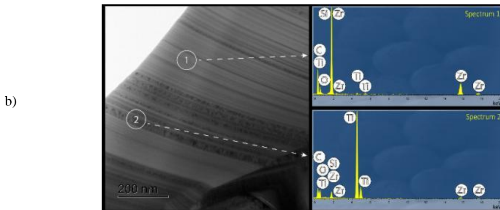
Fig. 4: Images of cross-sections of Zr-B-Si-C-Ti-N (a) and Zr-B-Si-C-Ti (b) coatings and characteristic EDX patterns from their various sections
