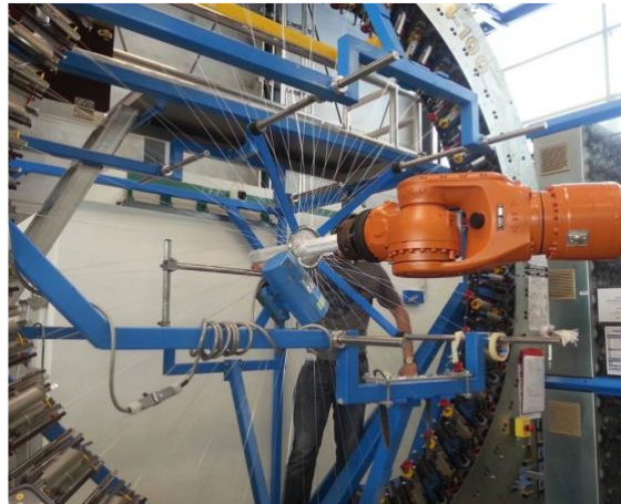
Fig. 1: Radial braiding machine with robotic arm which guides the mandrel.
