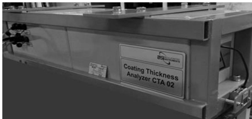
Fig.3. XRF gauge of CTA-02 analyser with optoelectronic displacement sensor (at the bottom of the frame on the right)
