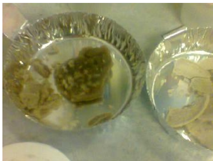
Figure 2: Extracted silica in Al pan ready for drying.
